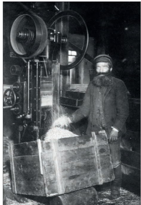
Fig. 18. A strip-cutting machine at the Rivne Match Factory. Photo by Solomon Yudovin
