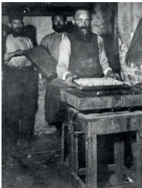
Fig. 21. A dipping pan at the Rivne Match Factory. Photo by Solomon Yudovin
